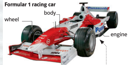
Did you know? Under a F1 car there's a plank of wood 10mm thick? At the end of a race, it shows that the car was not too low.
