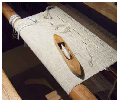
A shuttle on a weaving loom with a piece of woven cloth
